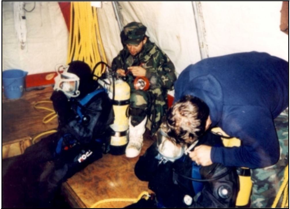
Figure 11-1. Ice Diving with Scuba. Divers in Typhoon dry suits and Aga/Divator FFM Scuba with approved cold-water regulators.
